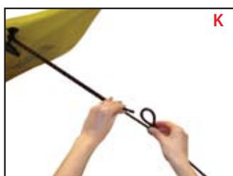
Thread the free end of the rope through the loop.
